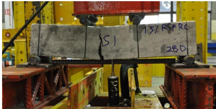
Figure 9: Failure mode of fibre reinforced concrete beam in flexure.
