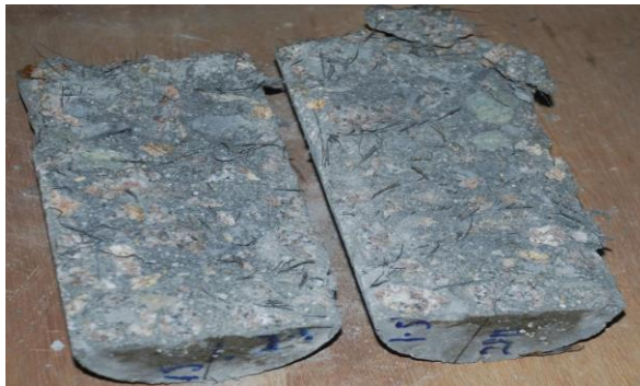
Figure 7: Distribution of steel fibre in broken cylinder.
