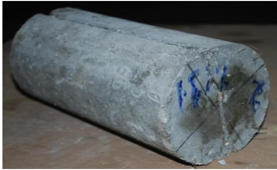
Figure 6: Concrete cylinder after splitting tensile test.
