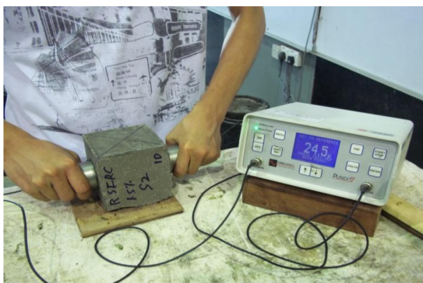
Figure 2: Testing of ultrasonic pulse velocity.
